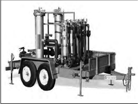
Pressurized Bag Filter (Source: http://www.dot.ca.gov )
